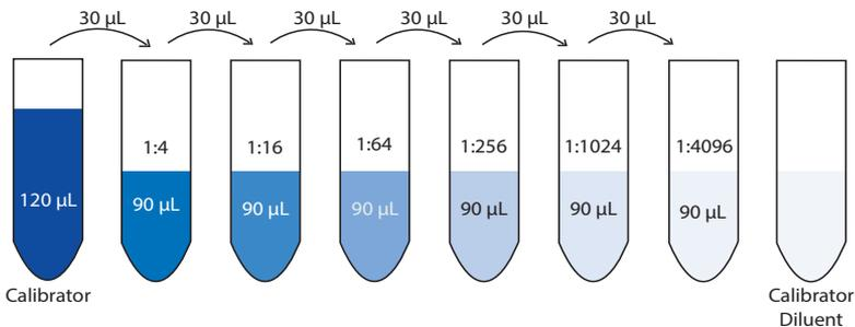
2. Prepare Samples: For the recommended sample dilution of 1:4, samples do not need any pre dilution. Samples that require further dilution should be diluted in calibrator diluent prior to diluting in complete assay diluent.
