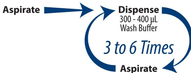
2. Ensure that the plate washer has a program that will not scratch the bottom of the microplate and will prevent plate drying. This is critical to prevent damage to the capture antibody arrays. The simplest method to avoid plate drying is to leave a small, uniform amount (1-3  $\mu\text{L}$ ) of wash in the well after the final aspiration, and add the next reagent to the plate as quickly as possible.
