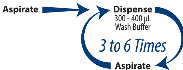
2. Ensure that the plate washer has a program that will not scratch the bottom of the microplate but will prevent plate drying. This is critical to prevent damage to the capture antibody arrays. The simplest method to avoid plate drying is to leave a small, uniform amount (1-3  $\mu\text{L}$ ) of wash in the well after the final aspiration, and add the next reagent to the plate as quickly as possible.
