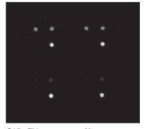
Q-View™ Imager generated image demonstrating typical sample results and reproducibility (samples shown were run in duplicates in each row). Samples can be run in duplicate or singlet allowing 45 to 90 unique samples to be run simultaneously on the same plate.
