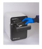
of the plate. Ensure there is no plate seal on the plate and there is only 1 plate on the tray. Press the eject button to close the tray and proceed to imaging.
