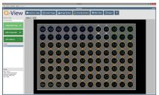
**3. Analyze & Export:** Q-View Software converts signal to concentration values. The optimal regression model is determined based recovery of the calibrator points. Includes highly customizable analysis reports that can be adapted to different LIMS platforms, as well as assay specific statistics to show the quality of the project.
